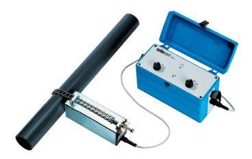
The Pipe Pecker simply connects to a pipe via a chain. The system then sends an acoustic pulse (knock) down the pipe at different frequencies depending upon the distance required. The noise from the pipe can be detected above ground by using a ground microphone. The system works particularly well on non-metallic potable water pipes such as asbestos cement, PE and PVC.
