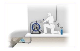
The PipeMic© uses a simple Bluetooth connection to either an external speaker or a set of headphones. The unit also contains a light bar to visually show the acoustic noise register all operated by a 9v battery.
