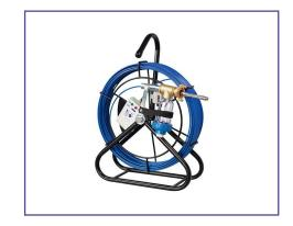
The PipeMic© uses a robust 4.5mm diameter rod which allows it to negotiate slow (long) radius bends in 25mm pipe. The rod has a rigidity that allows it to be used in smaller diameter mains up to 100mm in diameter.
