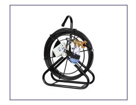
The PipeMic© Flex uses a unique ultra-flexible 4.5mm diameter rod which allows it to negotiate up to 3 x 90° short radius bends in 25mm pipe. The ultra-flexible rod has the fine balance between flexibility and rigidity to be able to push long distances. The 12mm diameter brass ball on the end helps to guide it through obstacles, fittings, and stiffeners.
