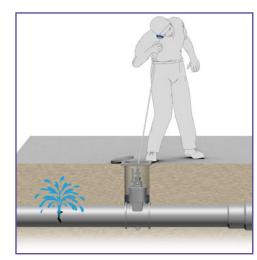
The FAST HMII is a robust listening stick manufactured from Steel and Aluminium. A silicone cover on the earpiece means that it is comfortable and easy listening stick to use.
